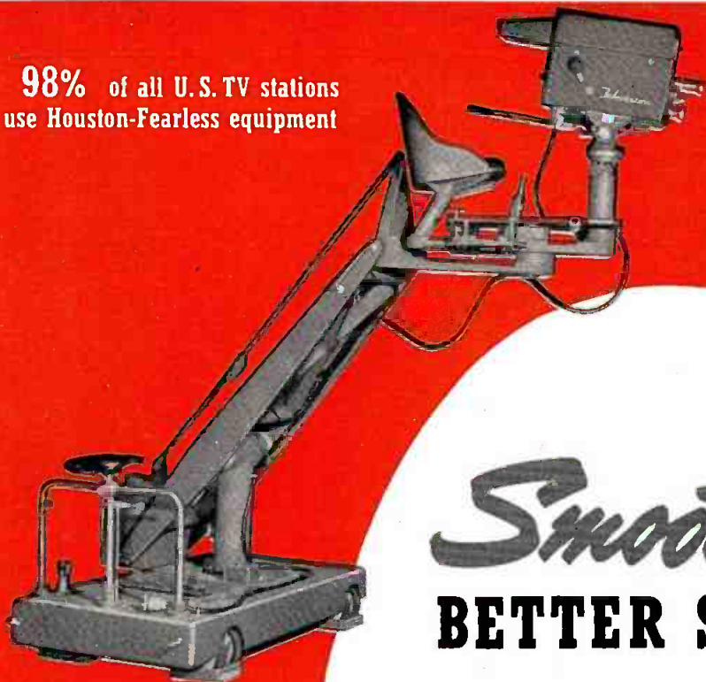
Houston-Fearless TV Crane, Model TC-1, offers extreme versatility. Camera lens can be raised quietly, from 3'-6" to 9'-6" while dollyling.
